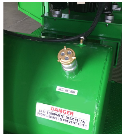
Fuel Tank - Open Side Door
